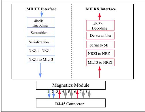
Figure 3. 82555 Analog Logic
